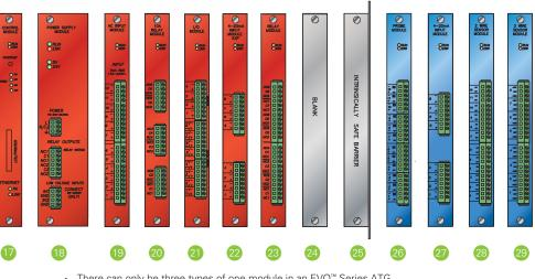
• There can only be three types of one module in an EVO<sup>™</sup> Series ATG.
